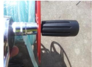
Left: Tighten bolt with washer into the end of the brass bush (note that flanged end at top goes into the reel housing)
