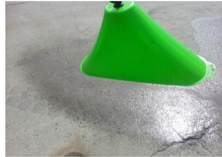
A useful spray guard can be attached to the lance in lieu of the adjustable cone-spray nozzle. The spray guard is an option
