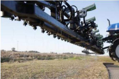
2. Clean the machine on the outside to prevent that the herbicide solution degrades sensitive materials<sup>[HB7]</sup>.
