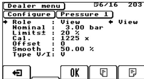
Mostly, a pressure sensor is a voltage sensor (V), not a current sensor (I). Smooth is 50.00% by default.
