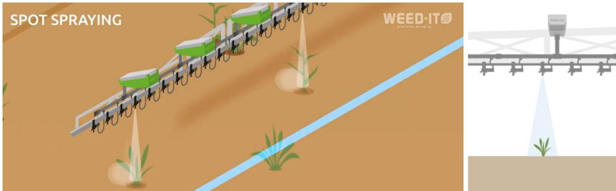
In Spot Spraying, the WEED-IT Quadro only sprays the green plants that are detected with the chlorophyll fluorescence principle. WEED-IT regulates the application rate via PWM, considering a constant pressure. The spot spraying application can be seen as a band application with a single nozzle. Therefore the spot spraying application rate is calculated as:
