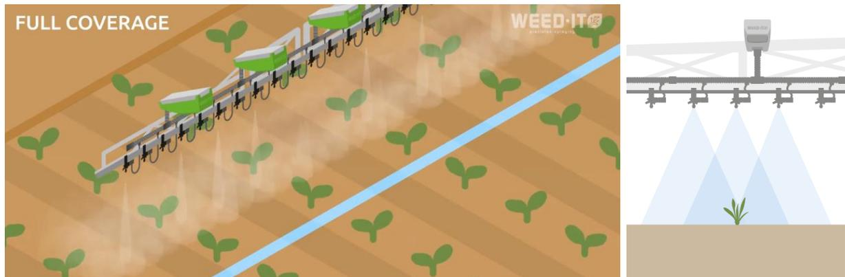
In Full Coverage spraying mode, the WEED-IT Quadro operates like a normal sprayer. The only difference is that the WEED-IT Quadro regulates the application rate via PWM, considering a constant spray pressure. The cover application rate is calculated as:
