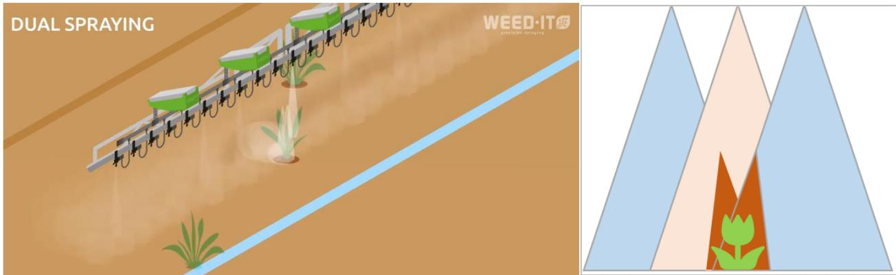
The Dual Spraying mode is a unique spray tech feature. It combines full coverage spraying with spot spraying by applying a low cover application rate, like 30 l/ha, followed by a spot application rate, like 100 l/ha, when a plant is detected. Unique is that both cover and spot application rates are regulated via PWM.
